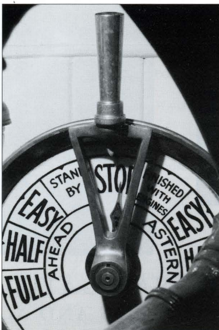
A Mason & Porter engine-room telegraph donated by Mrs L S Dromgoole in memory of the late Leo Dromgoole
