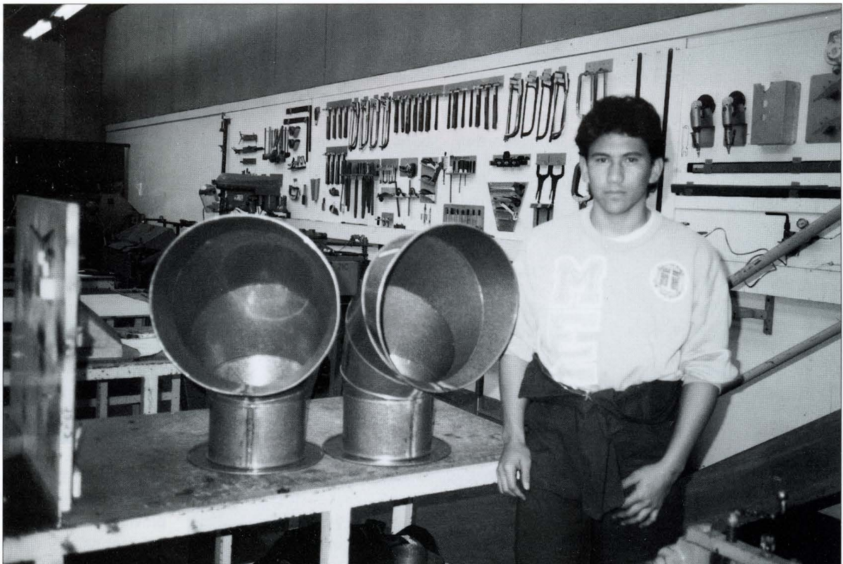
Kenneth Bedggood, a sheet metal fabrication student at Manukau Polytech, with the cowl vents he made under the supervision of Tutor Kelvin Baker, for the scow TED ASHBY. This support from Kenneth and Manukau Polytech is greatly appreciated
